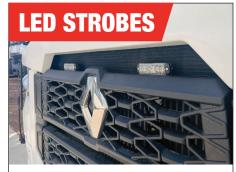
LED strobes to the front and rear, and two work lamps activated with reverse complete your lighting upgrades.
