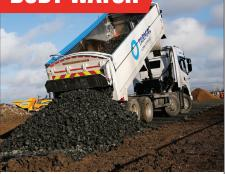
The body watch in cab and external detector is designed to alert the driver when moving off that the body of their tipper is still raised.
