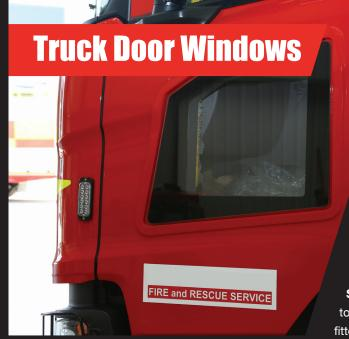
The truck door windows we fit are ideal for Direct Vision compliance and provide the truck driver visibility lower down the door on the left-hand side of the truck where Vulnerable Road Users (VRUs) often appear. Those installed by SM UK allow the passenger window to remain operable, unlike the factory fitted which are fixed window.
